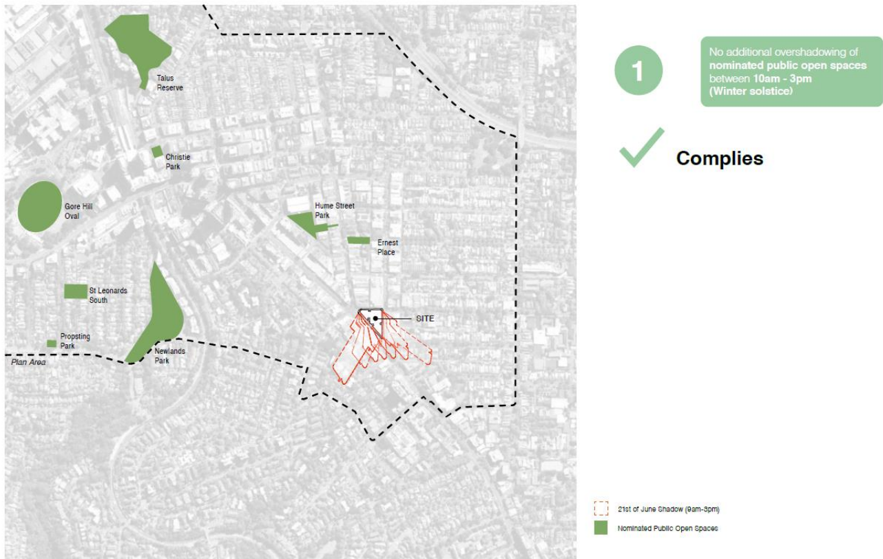
Figure 31: Shadow analysis - Impact on nominated public open spaces (Source: Turner - Urban design Report)
